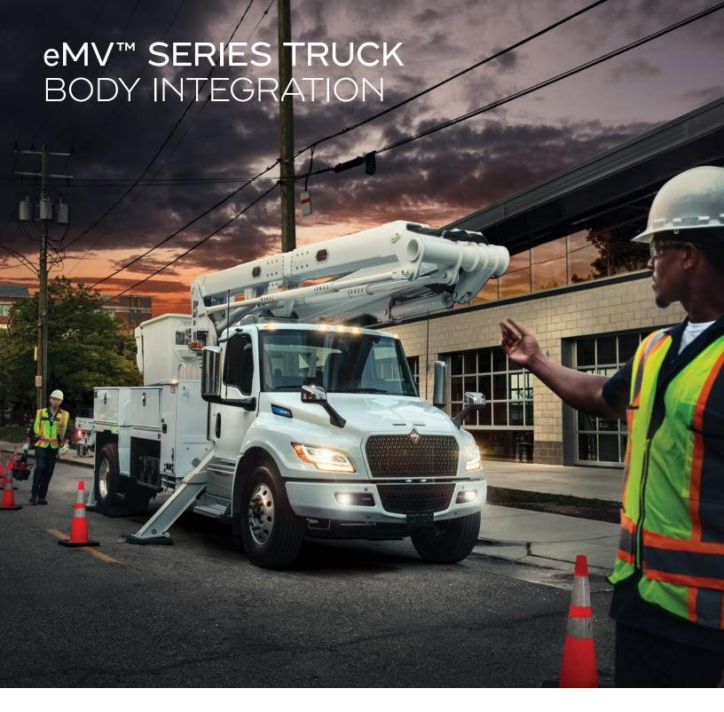
FACTORY-INSTALLED eMV™ SERIES TRUCK BODY POWER OPTIONS The International® eMV™ Series truck now offers ePower and ePTO options that use the propulsive batteries to power a wide range of body applications. From a simple plug in, to an electric motor with a SAE B flange, you now have the muscle needed to get the job done.
