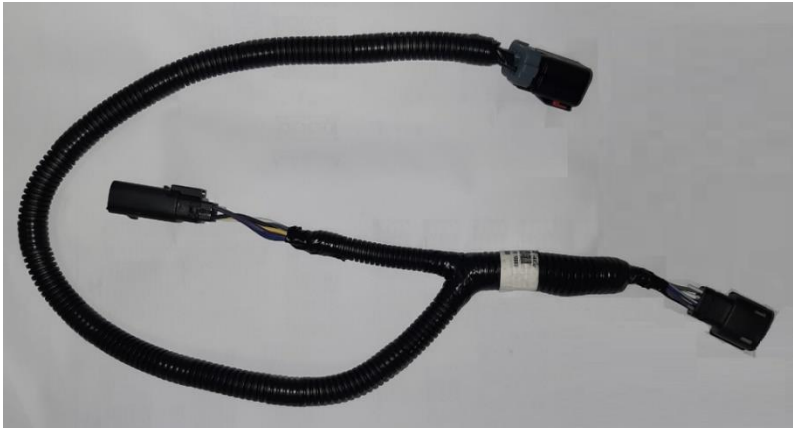
Figure 7.2.1.1: Y-Harness for Snowplow lights
